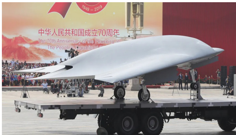
Figure 6: The new configuration of the Sharp Sword stealthy UAV (source: The Drive )
