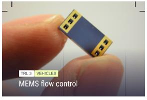
Micro flow control to eliminate control surfaces and reduce drag by 80%. Application to lifting surfaces and propulsion systems. Observability reduced
