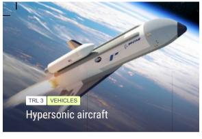
Trans-atmospheric vehicle with global radius. Allows rapid, reusable access to space and orbital payload insertion. May have combined-cycle propulsion (rocket/scramjet) with vertical takeoff
