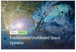
Provides redundancy, survivability and system upgradeability. Fractionation will involve system elements that cooperate and communicate via secure, jamresistant links (laser). Such systems are easily added to/repaired by adding or substituting small satellites.
