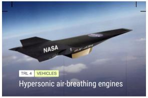
Propulsion technology and materials that can withstand the extreme temperatures of hypersonic flight will take another 20 years to develop. Automatic diagnostic and prognostic systems will allow reusable combined rocket/scramjet platforms for low cost orbital insertion. Inward turning inlets and dual flow paths will provide high volumetric efficiencies. Hypersonic transatmospheric aircraft to deal with heat issue as above Mach 10.
