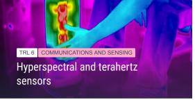
Stand-off detection of substances such as explosives and chemical agents. Improved imaging systems for vision through surfaces such as water, walls and vehicles. Multispectral sensor swarms.
