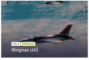
UAS accompanies a manned aircraft to conduct ISR, air interdiction, IADS attacks, offensive counter air, C2 of micro-UAS and provides additional weapons payload to the main aircraft. The wingman UAS can also be a transport or refuelling platform. Has embedded electronic EW (jamming) capability, self repair and diagnosis systems.
