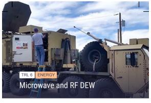
Delivery of electronic attack using directed energy to disrupt electronic components and personnel. Microwave beams will cause painful sensations with no lasting damage. RF attacks will damage electronics.
