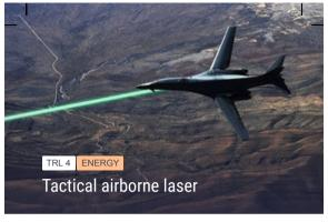
Use of solid-state and fibre laser systems to provide 300kW power and autonomous self defence against missile or aircraft threats. Possible tactical strike use.
