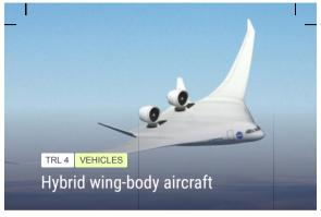
Highly unstable dynamically and requires fully automatic actuation and autonomous control under a variety of environmental conditions.
