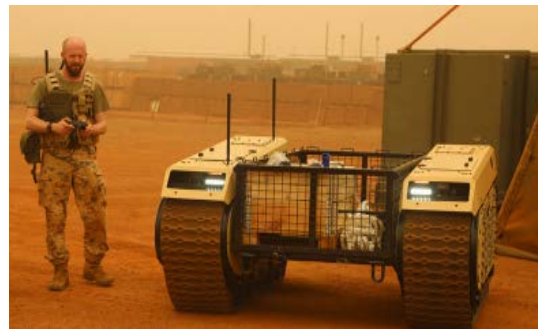
Figure 5: A Milrem Modular Unmanned Ground System (MUGS) being tested by Estonian troops in Mali. Source: mil.ee
