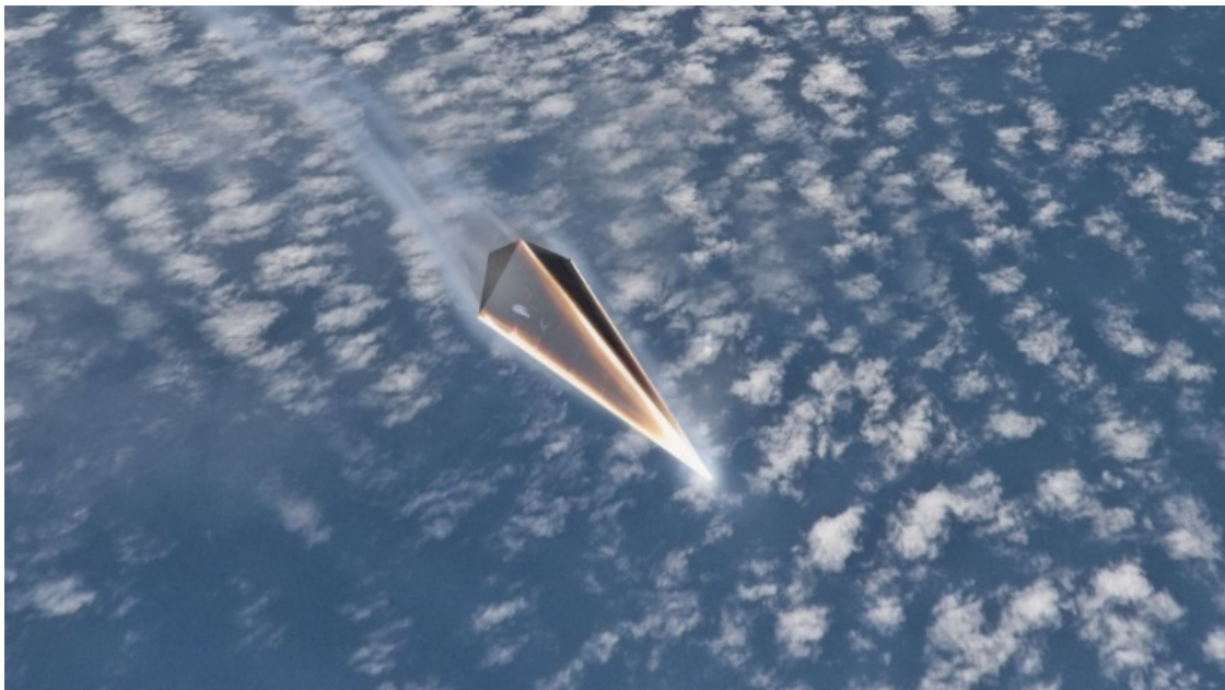
Figure 4: DARPA’s MACH programme will pursue materials and designs for cooling the hot leading edges of hypersonic vehicles travelling at speeds of Mach 5 and beyond (49)
