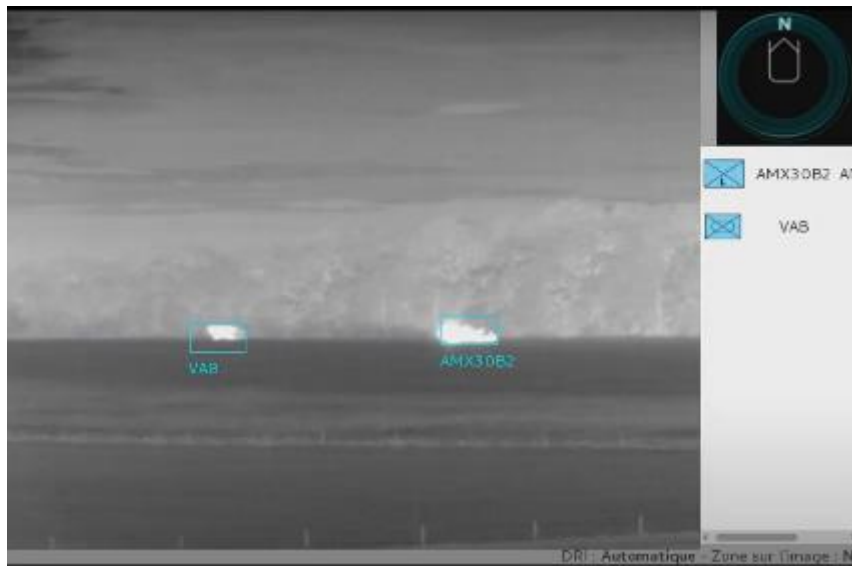
Figure 4: A screenshot of a 2ACI detecting and identifying vehicles taken from the MBDA YouTube announcement. The system was installed in a the turret sights of a French Army AMX10RCR tank. Source: MBDA
