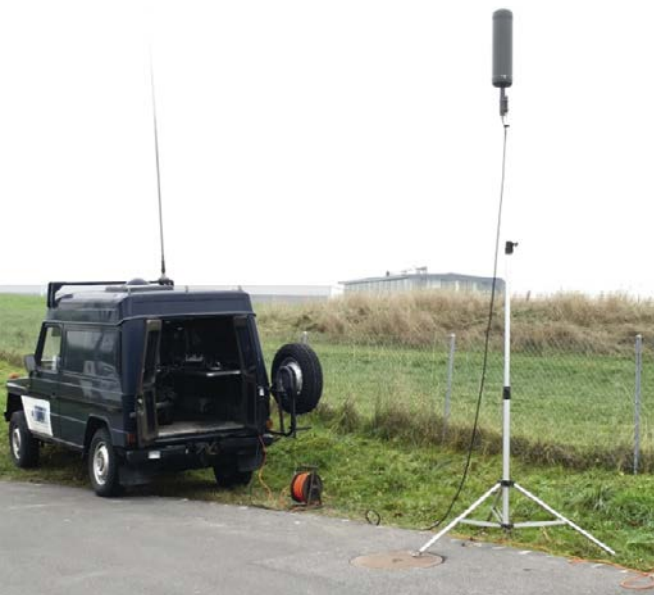
The measuring system can be installed in a Puch off-road vehicle specially equipped for measuring. It consists of a transmitter which emits a specially designed signal, and a mobile receiver station which measures all signal components and the delays in these.
