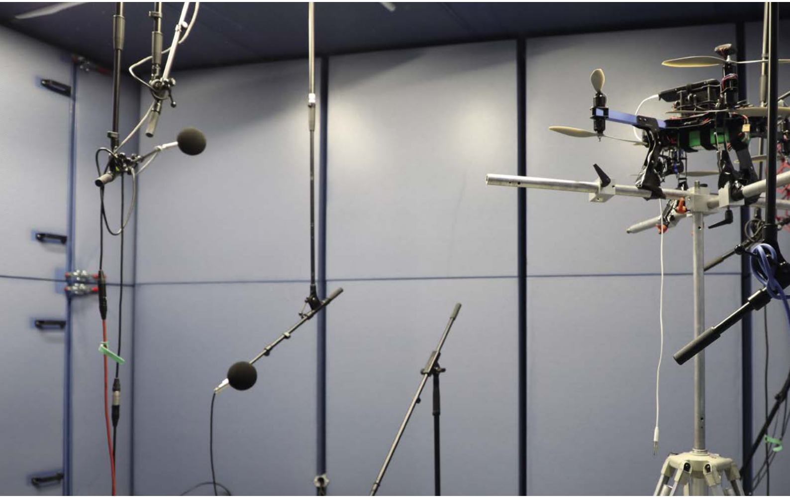
Partners are an important pillar of research for armasuisse. The picture shows an acoustics laboratory at research partner EMPA, where sensors are being measured to detect microdrones.
