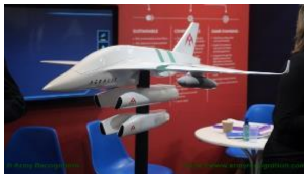
Figure 2: A model of the Aeralis modular military aircraft with the single and double engine modules hanging below the fuselage for demonstration purposes. Source: Army Recognition
