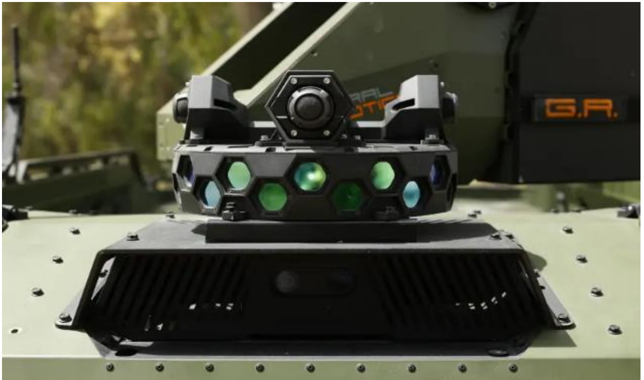
Figure 7: The OTHELLO-P gunfire detection system. Source: Israeli Aerospace Industries
