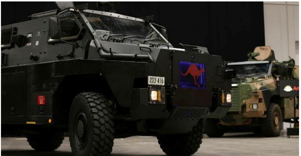
Figure 3: The US Army is not the only military organisation seeking to develop electric tactical vehicles. In August, the Australian Ministry of Defence revealed an electrical Protected Military Vehicle (e-PMV), also referred to as the electric Bushmaster, during the Chief of Army Symposium. The vehicle " brings the benefits of electric vehicles to the battlefield, being quieter than its combustion counterparts, and I look forward to seeing it perform in fields trials ", according to Australian Defence Assistant Minister Matt Thistlethwaite. Source: Australian Department of Defense
