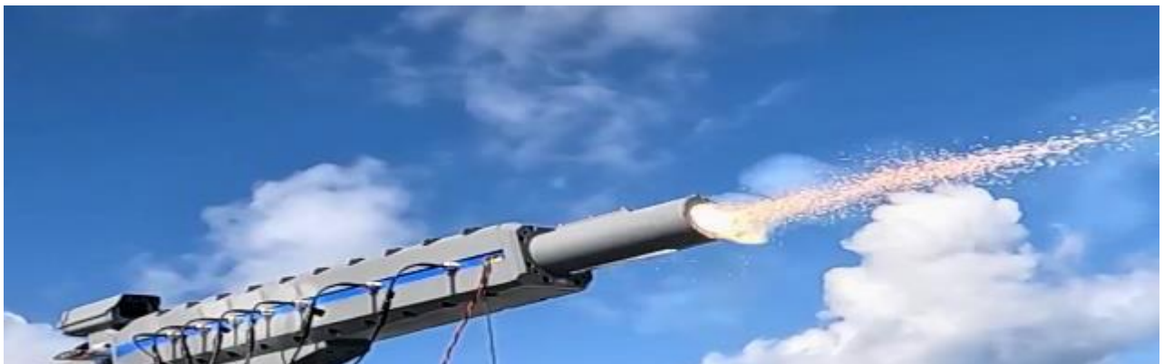
Figure 7: A screenshot from a video posted on ATLA's X account that shows the successful test of the maritime rail gun in October 2023. source: ATLA's X account
