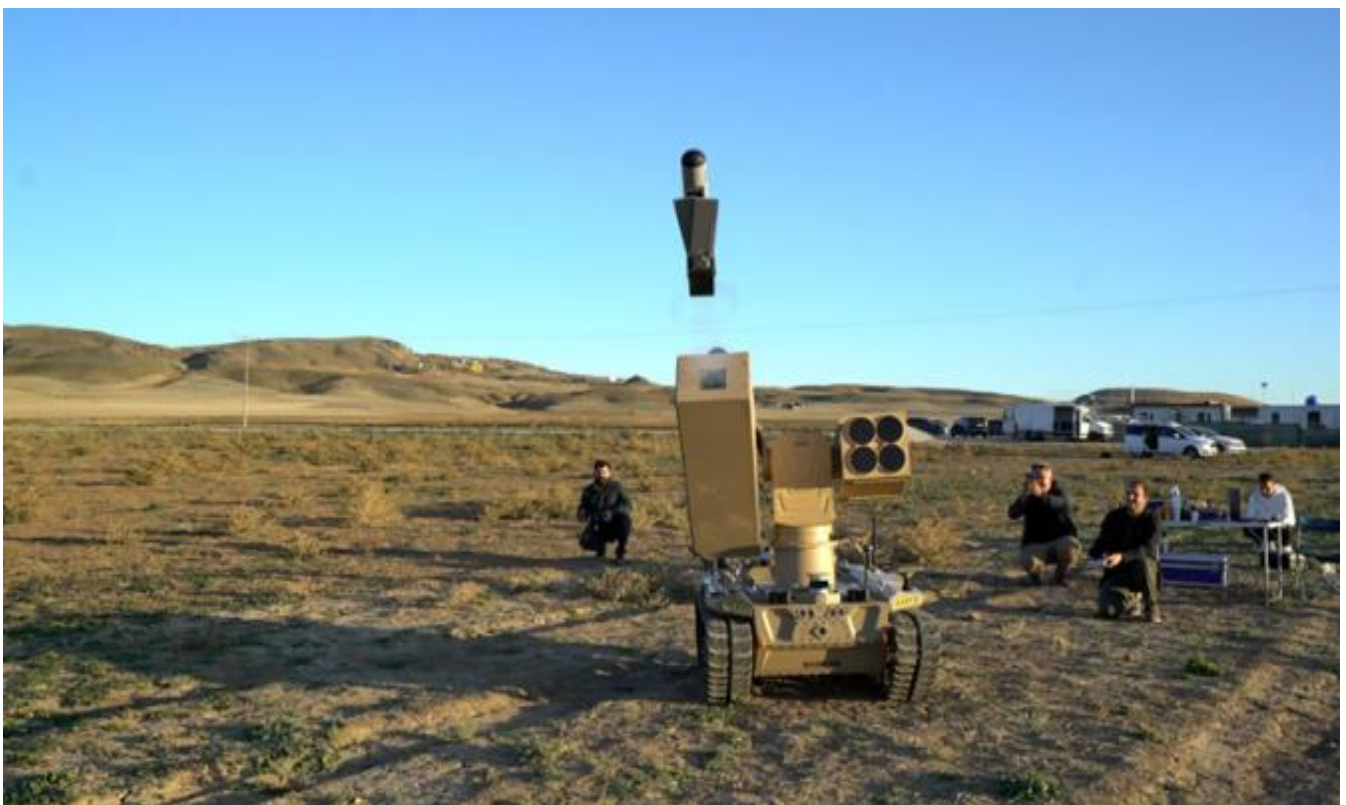
Figure 2: The Barkan 2 UGV launching a kamikaze drone during a recent test. Source: Havelsan
