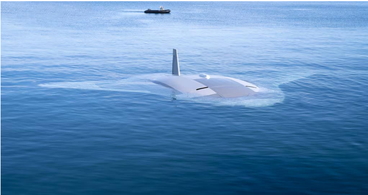
Figure 3: The Manta Ray UUV is a very large UUV capable of long-duration operations. Source: Northrup Grumman
