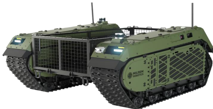
Figure 2: MILREM Robotics’ THeMIS modular UGV. Source: MILREM Robotics
