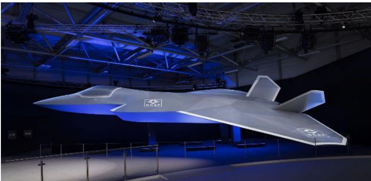
Figure 2: The new GCAP design displayed at the Farnborough Air Show in July 2024. The new design features a delta wing design and much larger wingspan than previous versions. Source: BAE Systems
