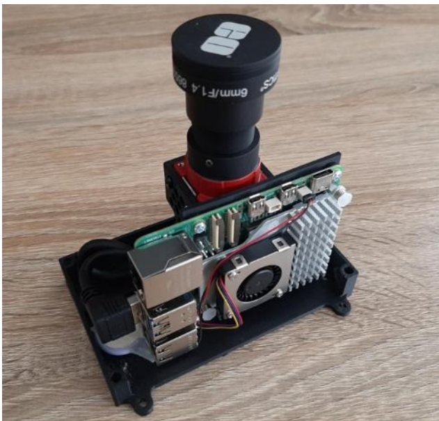
Figure 3: An image of the celestial payload (left), consisting of a Raspberry Pi 5 and an Alivium 1800 U-240 monochrome sensor fitted with a 6 mm f/1.4 wide angle lens, and the layout of the autopilot and celestial payload on the drone used during the 72-minute test flight. Source: Original research paper
