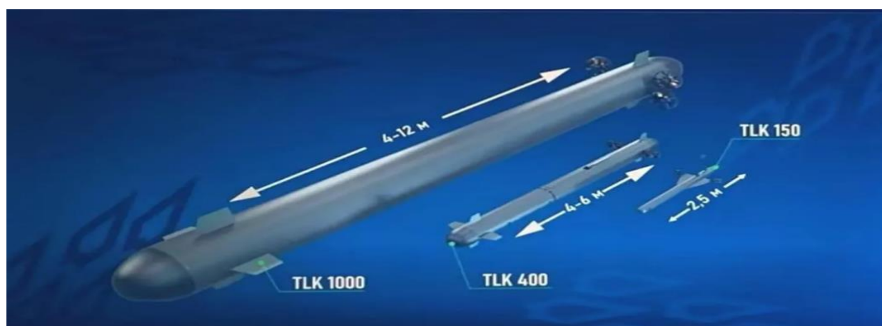
Figure 3: The relative dimensions of the Toloka series of uncrewed maritime vehicles. Source: Toloka
